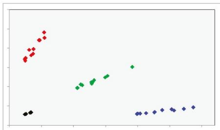
Results from the KASP trial kit reaction plate when run on the QIAGEN Rotor-Gene Q instrument using the standard KASP thermal cycle. Data has been exported and plotted using the scatter plot function in MS Excel.
