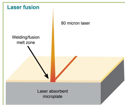
Our patented Fusion<sup>3</sup> plate sealer<sup>1</sup> is a fully automated benchtop instrument that uses a directed laser beam to quickly “fuse” seals on to flat-top microplates. It has the flexibility and precision to seal plate densities from single well reservoirs to 3456-well format.
