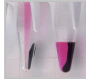
When removing supernatants it is important to remove as much of the liquid as possible without dislodging the particle pellet. With magnets used for manual protocols the particle pellet forms on the back wall of the sample tube. When placing the pipette tip inside the tube be sure to aim the end of the tip to the front wall of the sample tube to avoid disrupting the particle pellet.
