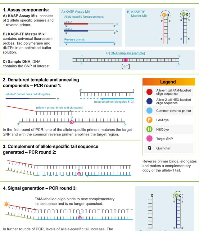
Fluor labelled part of the FRET cassette is complementary to new tail<br/>sequences and binds, releasing the fluor from the quencher to generateFluor for incorporated<br/>G allele no longer<br/>quenched.Fluor for non-incorporated<br/>T allele remains<br/>quenched.
