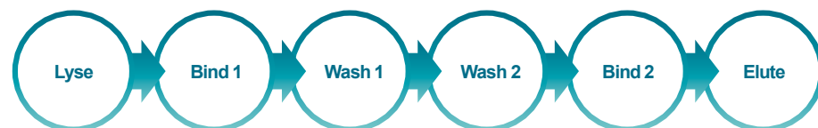
Figure 1. Easy 6-step purification procedure using Biosearch Technologies' innovative sbeadex technology.
