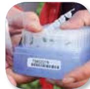
1. Once the 96-well storage rack is full (or all required plants have been sampled), seal each strip of tubes within the rack using the perforated strip caps provided. Press each cap firmly into place to ensure that the tubes are securely sealed.
