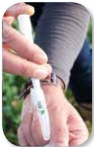
4. Insert the end of the cutting tool into the first well of the 96-well tube storage rack and depress the plunger to dispense the leaf disc. Please note: the tubes are in strips of 8 and can be lifted out of the rack to aid dispensing of the leaf disc.
