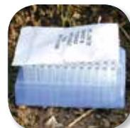
3. Place the desiccant sachet directly on top of the strip capped tubes.
