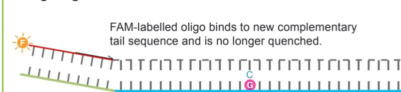
In further rounds of PCR, levels of allele-specific tail increase. The fluor labelled part of the FRET cassette is complementary to new tail sequences and binds, releasing the fluor from the quencher to generate a fluorescent signal.
